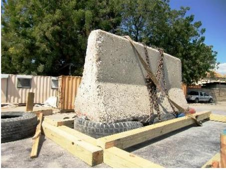
We then built a solid wooden frame at the Haiti Communitere workshop to keep the tires in place on the truck. The concrete weight was a road separation block weighing over 1.1 ton, which corresponds to a house wall on top of three tires in a row.
